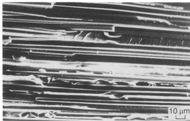
Figure 3 Scanning electron micrograph of CTU4/PTI (B) fracture surface.
